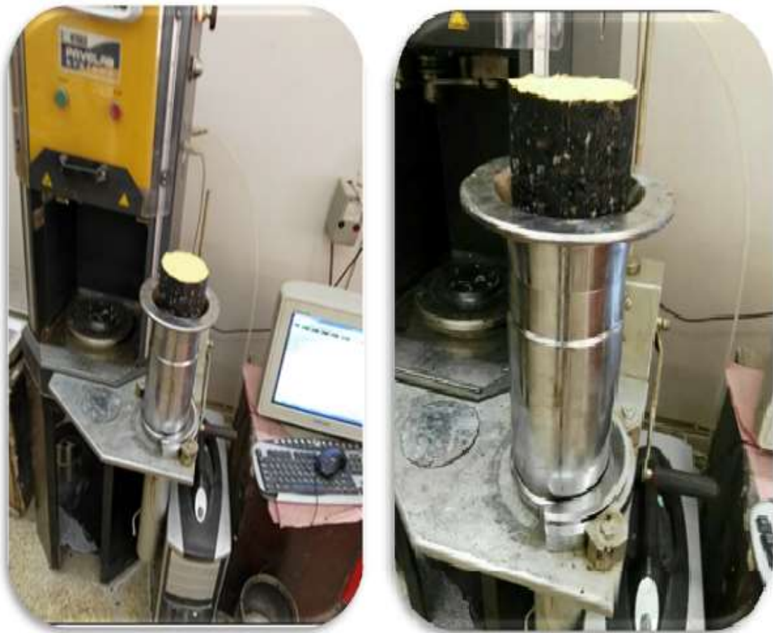
Figure (3-11) Equipment of Superpave gyratory compacter.
