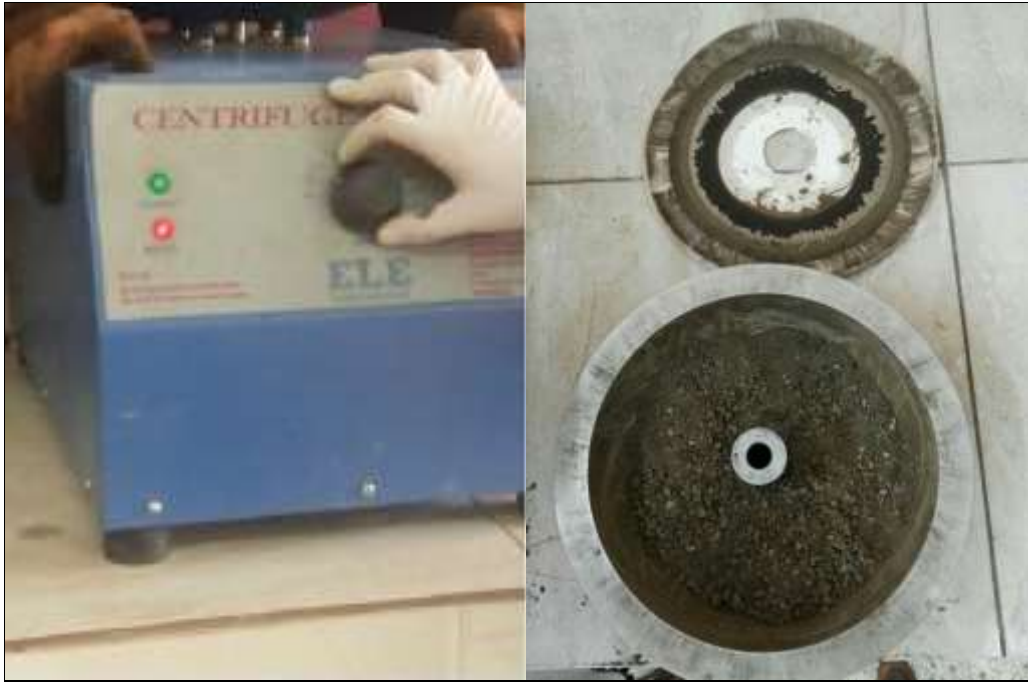
Figure (3-12) Extraction test procedure.
