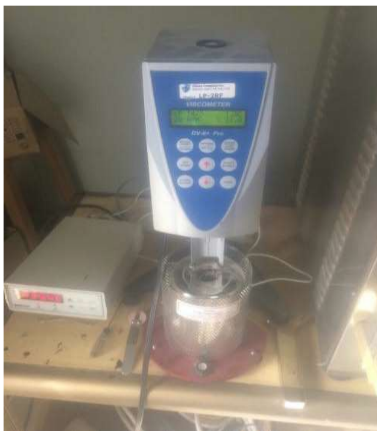
Figure (3-6): Rotational viscometer device at Al-Nahrain University.
