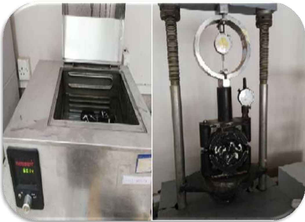
Figure (3-13) Marshal Test procedure at University of Technology.
