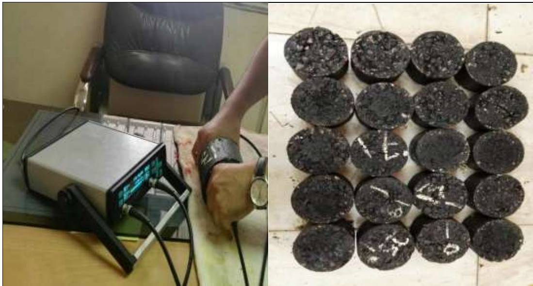
Figure (3-16) Ultrasonic testing device and samples.
