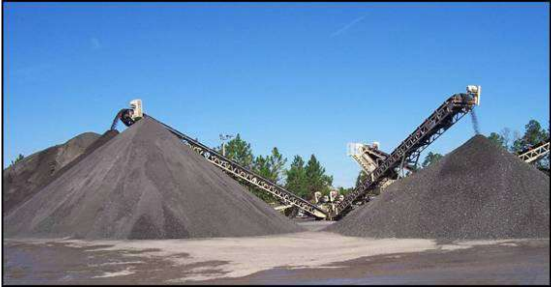
Figure (1.1): Pavement Recycling with Reclaimed Asphalt Pavement (RAP), (Kennedy et al. 1998).
