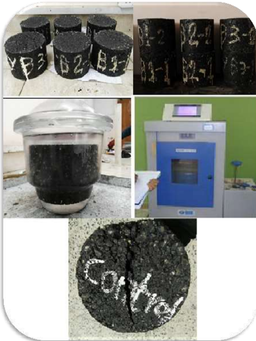
Figure (3-10): Apparatuses used in indirect tensile strength test.
