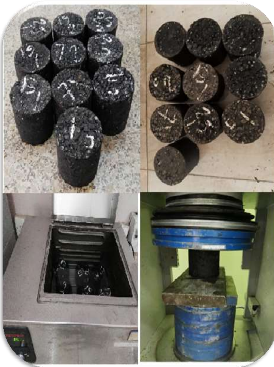
Figure (3-15): Compressive strength test University of Technology.
